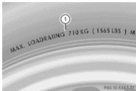
Maximum tire load **1** is the maximum permissible weight for which the tire is approved.
