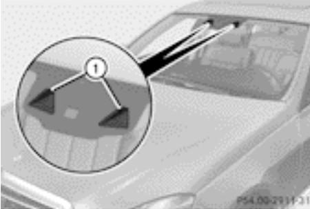
Active Lane Keeping Assist monitors the area in front of your vehicle by means of camera system ① at the top of the windshield.
