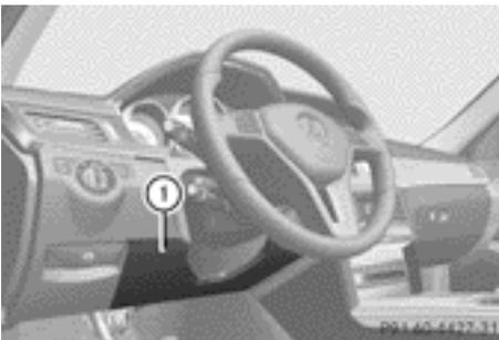
Driver's knee bag ① deploys under the steering column. It is deployed together with the front air bags. The driver's knee bag is designed to operate together with the front
