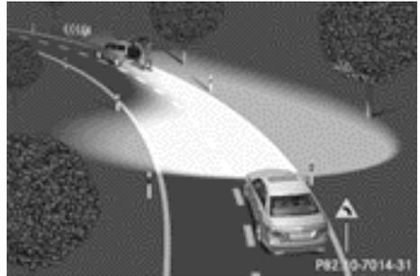
The active light function is a system that moves the headlamps according to the steering movements of the front wheels. In this way, relevant areas remain illuminated while driving. This allows you to identify pedestrians, cyclists and animals.
