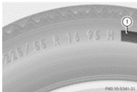
In addition to the load bearing index, load index **1** may be imprinted after the letters that identify speed index **6** on the sidewall of the tire (▷ page 389).
