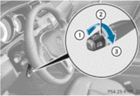
You can set the specified minimum distance for DISTRONIC PLUS by varying the time span between one and two seconds. With this function, you can set the minimum distance that DISTRONIC PLUS keeps to the vehicle in front, dependent on vehicle speed. You can see this distance in the multifunction display (▷ page 197).
