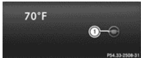
If DISTRONIC PLUS Steering Assist is activated but is not ready for a steering intervention, steering wheel symbol **①** appears in grey. If the system provides you with support by means of steering interventions, symbol **①** is shown in green.
