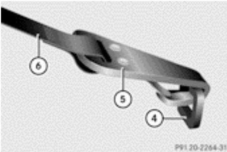
The Top Tether anchorages are attached to the rear of the rear seat backrests.
